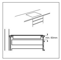
If the appliance is installed above a drawer, the hob ventilation can warm up the items stored in the drawer during the cooking process. You can instal a separation panel but it is not mandatory.
