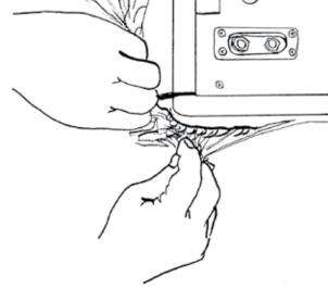
**C.** Peal the clear protective film away from the attachment surfaces on the piano bottom.
