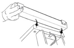
**B.** Locate the 2 holes in the stand leg bottom. This is where you will thread in the screws that are already in the feet.
