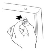
**B.** On the outside of the stand leg tops, locate the 4 large holes where the cam locks will be inserted.
