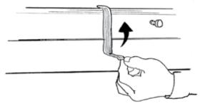
**B.** After you have placed your piano in your home, now remove all the clear protective film and the fiberglass tape holding the fallboard in place.
