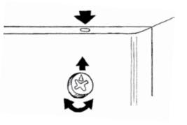
**C.** The cam locks have a Phillips head X with a small arrowhead. Slide the cam lock into the stand hole with the Phillips head facing out and the arrow pointing up towards the small hole in the top of the stand.
