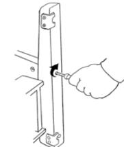
**D.** Push the screws into the holes in the feet and align them to thread into the stand barrel nuts. Make sure the pads mounted on the bottom of the feet face to the inside of the stand before you tighten the feet screws.
