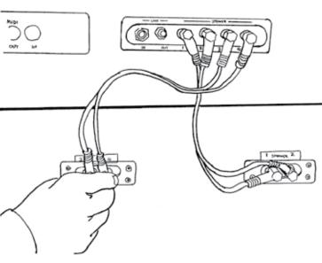
**G.** Locate the speaker connection cables. They have red and white 1/4" male plugs. On the back of the piano locate the receptacles marked speaker 1 2 3 4 and on the back of the stand locate the 2 dual receptacles marked (3 speaker 4) and (1 speaker 2). Using the connecting cables connect the matching numbers i.e. 1 to 1, 2 to 2, and so on.
