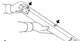
**A.** Remove the clear protective film from the stand feet. You will notice the attaching hardware is already in place.
