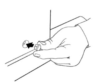
**H.** Locate the 8 large cover caps and push them into the large barrel nut holes on the outside of the stand legs.
