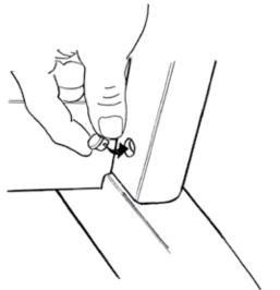
**1.** Locate the 4 small cover caps and push them into the small barrel nut holes on the inside bottom of the stand leas.
