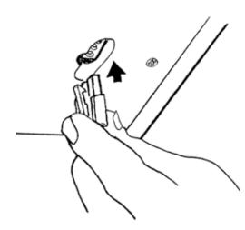
**F.** Under the right front of the keyboard locate the pedal control plug. It is coming out of the top front of the right stand leg. Plug it into its receptacle on the bottom of the piano.
