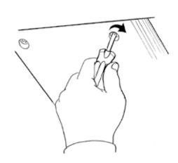
**E.** With the piano rods seated in the cam locks, rotate the cam locks clockwise 3/4 of a turn.
