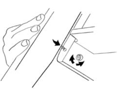
**C.** Go to the inside of the stand lea and locate the barrel nuts already in their holes. Notice the barrel nut has a Phillips head X in it as well as a large straight slot. Align the straight slot to point to the intersecting hole in the leg bottom. This will align the threads in the barrel nut with the intersecting hole and the feet screws.
