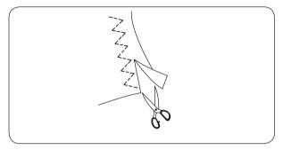
This stitch is used to finish the raw edge on synthetics and other fabrics that tend to pucker. Place your fabric to allow a 1.6 cm (5/8") seam. Trim the seam allowance after sewing. Be careful not to cut the stitches.
