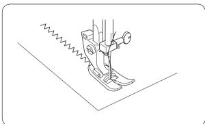
Simple zigzag stitching is widely used for overcasting, sewing on buttons, etc.
