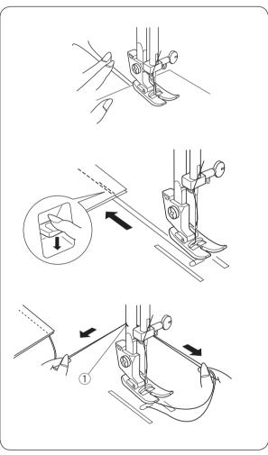
with its edge lining up with a seam guide line on the needle plate.
