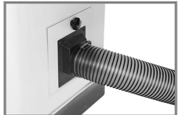
Figure 35. Dust hose attached to dust port.
