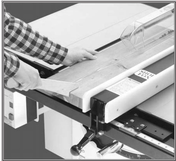
Figure 53. Typical ripping operation.
