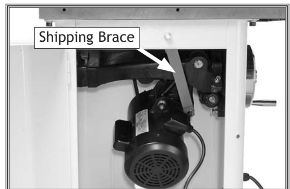
Figure 13. Shipping brace location.
