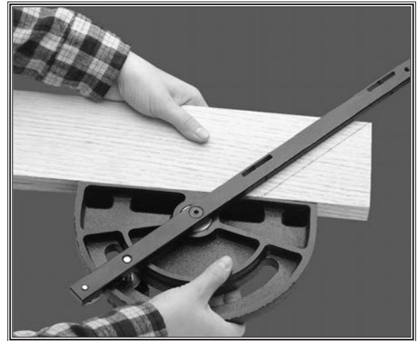
Figure 55. Example of marking miter line.
