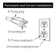
AWARNING —Improper use of the grounding plug can result in a risk of electric shock. Do not use an extension cord. If the power supply cord is too
