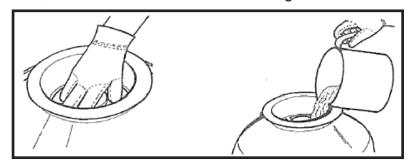
**4.** Remove the funnel and make sure the tanl's neck is clean. Put the O-ring on the valve and use clamp to fix the valve with the tank. Pump port valve direction needs to face pump's out-port.
