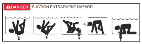
POOL AND SPA PUMPS MOVE LARGE VOLUMES OF WATER, WHICH CAN POSE EXTREME DANGER IF A PERSON;S HAIR COMES IN PROXIMITY TO A DRAIN THAT IS NOT THE PROPER SIZE FOR THE PUMP OR PUMPS.
