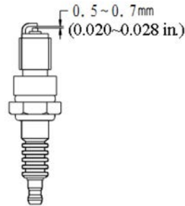
Figure 9 Measuring the spark plug gap
