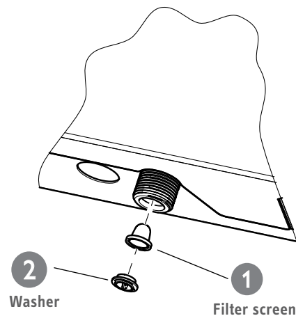
Filter screen location in Tempra® models
