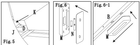
Fig.5: Extend the Small Canopy (K) onto the small top by fixing the canopy at four corners of top.
