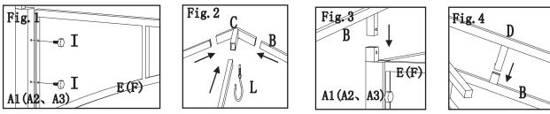
Fig.1: Attach the Long Screen (E) and the Short Screen (F) to Post (A1、A2、A3) with the Bolt (I).
