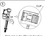
Slide tab in the "Open" direction as shown in the drawing.
