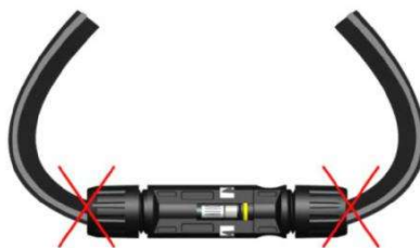
Incorrect Routing of cable
