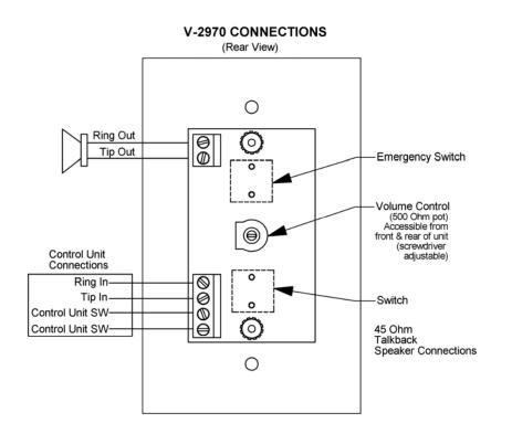
**NOTE:** When utilizing the V-2970 volume control with 45 Ohm talkback speakers featuring an integrated volume control or volume preset capability, set the volume at the speaker to maximum. This will allow full volume range from the V-2970 volume control.
