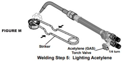
**14.** Open the acetylene control valve (B8 and AC label B10) about a 1/4 turn and ignite the acetylene gas coming out of the nozzle (part D3, D6) **Always point the nozzle away from other people when lighting**.
