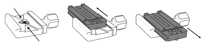
A 3rd Party Clamp Warning: Our safety stop screws work with most 3rd party quick-release clamps, but clamps that do not have channels and are too wide to be straddled by the safety stop screws will not work.
