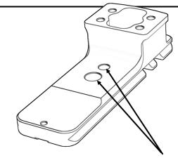
Using the AP-600 without using a quick-release The 3/8 and 1/4 inch holes in the middle section of the plate can be used to attach the foot directly to the threaded stud of a monopod or other lens support equipment, without needing a quick-release clamp.
