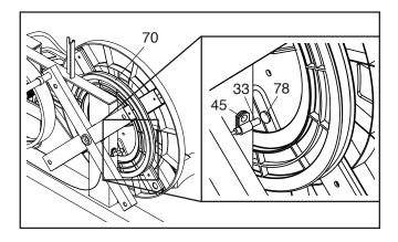
Next, rotate the Pulley (70) until the Magnet (78) is aligned with the Reed Switch (33). Slide the Reed Switch slightly toward or away from the Magnet. Then, retighten the M4 x 20mm Self-tapping Screw (45). Rotate the Pulley for a moment.
