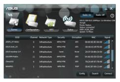
**SSID** - Displays the name of the wireless network that the WLAN adapter is connecting to.
