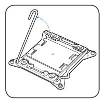
Press the right load lever with your thumb (C), then move it to the right (D) until it is released from the retention tab. Lift the load lever in the direction of the arrow (E).
