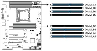
Z9PA-U8 240-pin DDR3 DIMM sockets
