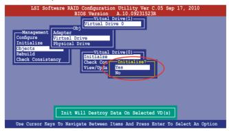
5. A progress bar appears on the screen. If desired, press <Esc> to abort initialization. When initialization is completed, press <Esc>.
