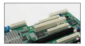
2. Align the golden fingers of the PIKE RAID card with the PIKE RAID card slot.
