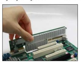
3. Insert the PIKE RAID card into the PIKE RAID card slot. Ensure that it is completely seated on the PIKE RAID card slot.
