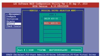
After selecting the drive to rebuild, press <F10>. When prompted, press <Y>
