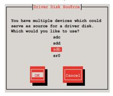
6. Insert the Red Hat® Enterprise RAID driver disk to the USB floppy disk drive, select **OK**, then press <Enter>.
