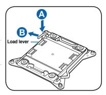
3. Slightly lift the load lever in the direction of the arrow.
