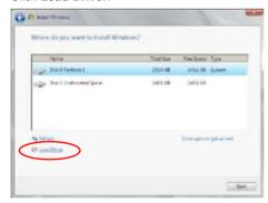
4. A message appears, reminding you to insert the installation media containing the driver of the RAID controller driver. If you have only one optical drive installed in your system, eject the Windows OS installation disc and replace with the motherboard Support DVD into the optical drive. Click **Browse** to continue.
