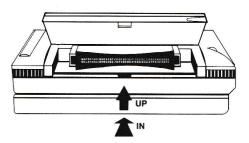
Turn the Portfolio and the Memory Expander Plus right side up. Slide the Memory Expander Plus into the bus connector as shown below until there is an audible click from the retaining clips.
