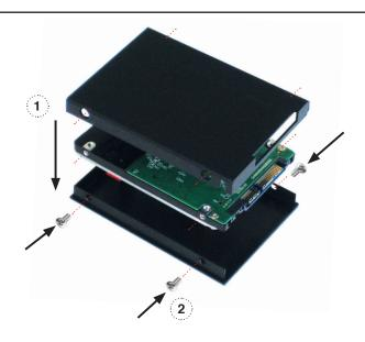
(1) Important: Insert screws last and DO NOT over-tighten the screws or proper alignment of the Master Caddy can not be guaranteed.
