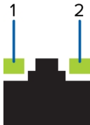
Figure 2: (1) Link LED. (2) Connection activity LED.
