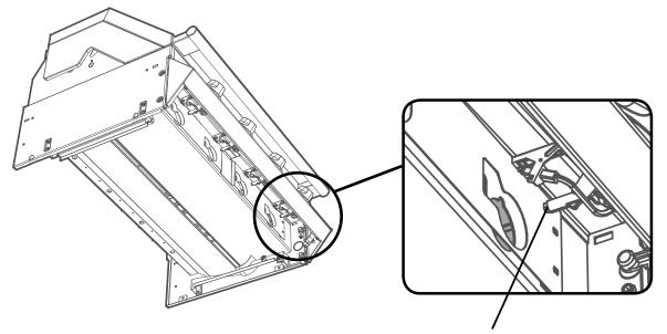
Unscrew the LPG injectors and replace with natural gas injectors on all valves. All injectors are marked with the orifice size Remove LPG injector and install injector for natural gas
