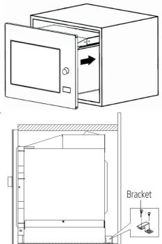
2. Open the door, fix the oven to the cabinet with Screw through the installation hole. Then fix the trim-kit plastic cover to the installation hole.
