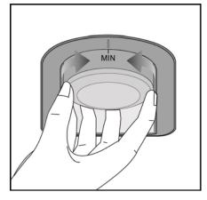
Operating temperatures are controlled by the thermostat knob (see diagram) located on the ceiling of fridge compartment. Settings may be made from **MIN**, 1 ... **MAX**, **MAX** being the coldest position.
