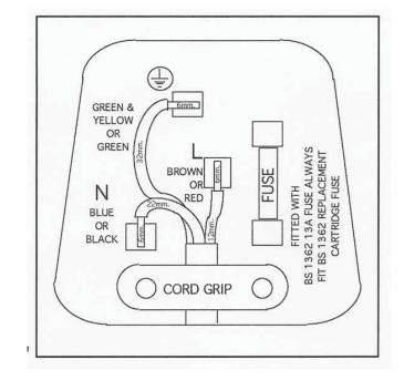
With alternative plugs a 13 A fuse must be fitted either in the plug or adaptor or in the main fuse box.
