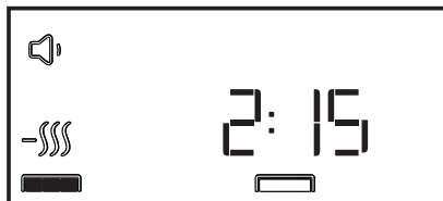
Drying level damp
