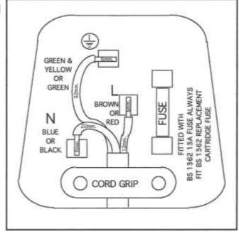
With alternative plugs a 13 A fuse must be fitted either in the plug or adaptor or in the main fuse box.
