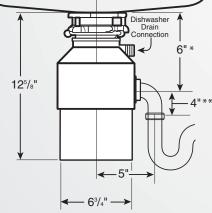
Distance from bottom of sink to center line of disposer outlet. Add 1/2" when stainless steel sinks are used.
