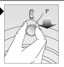
Attention! Keep the safety bolts for future transportation and reinstate them before transporting your machine. Never transport your machine without the transport bolts in position. Any resultant damage is not covered by the warranty.
