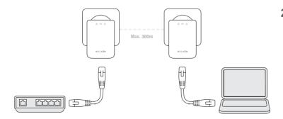
2. Connect one of the Adapters to your existing modem or router with a network cable. Use a second network cable to connect the other Adapter to an Internet TV, Blu-ray® player, computer, or other network device such as a wireless access point, set-top box, or gaming console.
