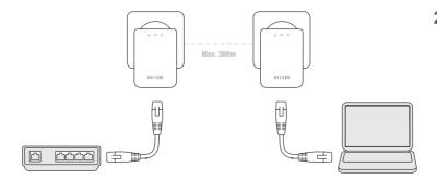
2. Connect one of the Adapters to your existing modem or router with a network cable. Use a second network cable to connect the other Adapter to an Internet TV, Blu-ray® player, computer, or other network device such as a wireless access point, set-top box, or gaming console.
