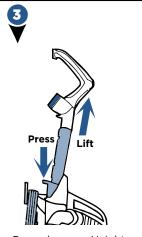
Press down on Height Adjustment Lever and pull out Handle.
