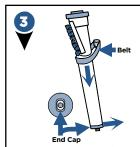
Replace roller and/or belt. To reassemble roller, thread through belt and line up End Cap, then place bottom cover back on and replace 7 screws.
