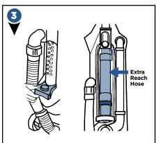
Snap lower cord wrap to lower back of unit. Attach extra reach hose to back of unit. Wrap power cord.
