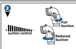
Twist counter-clockwise to reduce suction for drapes, delicate surfaces, or thick/plush carpet, etc.
