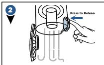
Holding Dirt Container over a trash bin, press Release Button on back.
