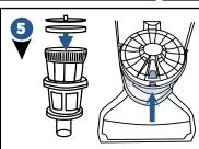
Place dry pre-motor filters back on top of dirt container with black tabbed side on top. Place post-motor filter back to bottom front of vacuum and snap filter cover door back on.
