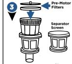
Remove pre-motor filters and check for dirt on BOTH sides. Separator Screen can be rinsed and dried as well.
