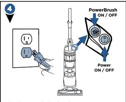
Plug into a polarized outlet
