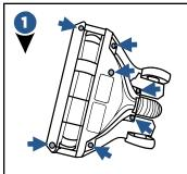
Unplug vacuum, turn over and unscrew 7 Philips head screws to remove bottom cover
