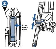
Pull Extra Reach Hose off back of vacuum and insert into Main Hose connection.
