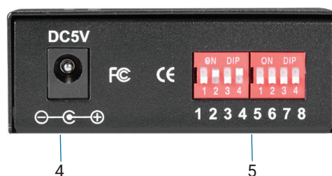
FIGURE 2-4. LHC211A BACK PANEL
