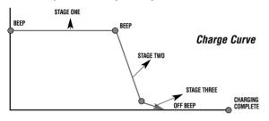
**Stage Three** — Top-Off Charge voltage is automatically maintained and reduced to a predetermined level while current is adjusted for a safe, effective battery charge. At the end of Stage 3, the unit will BEEP signaling the completion of the charging cycle.
