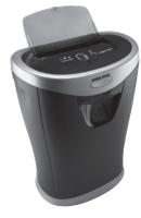
Sheet capacity: 12 20 lb. pages in one pass Paper shred size: 5/32" x 2" 4mm x 50.8mm Maximum running time: **15 minutes** Automatic cool-down period: 30 minutes Voltage: **120**
