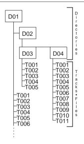
Each directory can be given a name using a PC. The device is capable of displaying the directory name. You should name the directories and tracks/files using the method provided by your CD burner software. The software's instruction manual will provide details on how to do this.
