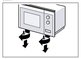
Secure the built-in frame on the microwave base with the two outer screws.
