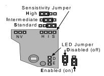
**Standard:** Tolerates most environment extremes on this setting, but requires the largest amount of intruder motion to achieve an alarm. Standard Sensitivity is not recommended for use with barrier, long range barrier or dual corridor coverages.
