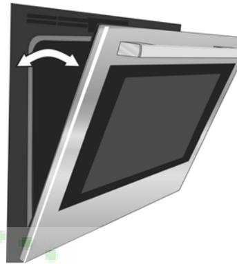
4. Close the oven door until it catches on the hinge stop levers. The door will be open about 7 inches at the top. This takes the spring tension off the hinges so the door can be easily lifted out.
