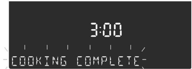
This screen remains in the display until it is cleared by pressing the **Oven Clear/Off** touchpad or until the probe is removed. The display then goes back to stand by mode.
