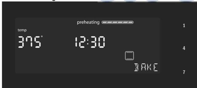
**Note:** If a temperature is entered that is not within the allowed range for the mode an error tone will sound and the lower part of the screen will display “TEMP NOT ALLOWED”.
