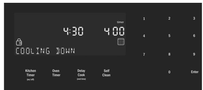
6. When the cool down is complete, the message **"SELF CLEAN FINISHED"** is displayed. Continue to use caution when opening the oven door.
