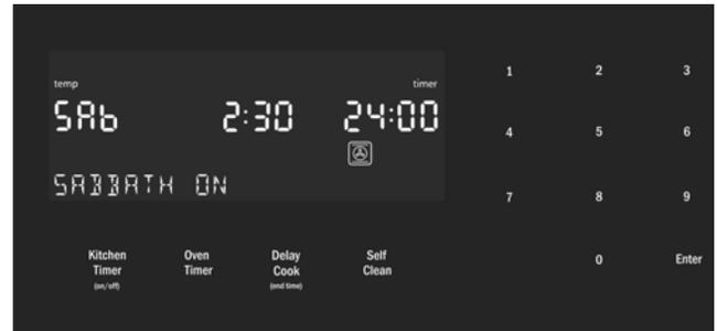
4. After the Sabbath mode countdown reaches zero, the oven displays the current time and the message "SABBATH". No user input is accepted in this state. To end the Sabbath Mode and return to normal function, press the **Oven Clear/Off** touchpad.
