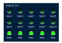
In the event of an alarm, the green alarm LED for the triggering alarm input appears next to the video image. The unit's configuration determines whether the alarm is displayed, as well as additional details (see **Livepage configuration**, page 112).
