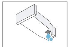
Check the condensation container filter → Page 44 regularly and clean the filter if it is dirty. Make sure that you insert the condensation container before operating the appliance.
