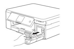
Open the ink cartridge cover, and then remove the orange protective part from the machine.
