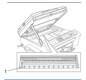
Clean the machine printer platen (1).
