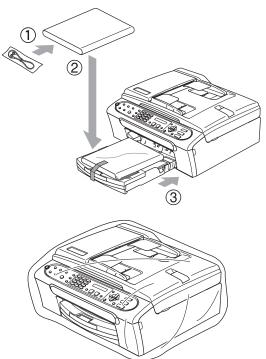
12 Pack the printed materials and additional parts (handset and cords) in the original carton as shown below. Do not pack the used ink cartridges in the carton.
