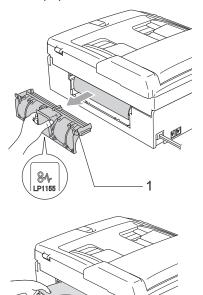
5 Put the Jam Clear Cover back on. Make sure the cover is set properly.
