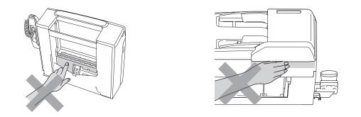
When moving the machine you must lift it from the base, by placing a hand at each side of the unit as shown in the illustration. Do not carry the machine by holding the scanner cover.
