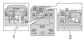
Press the tab (1) and place the front of the cradle in position.
