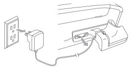
Using both hands, use the plastic tabs on both sides of the machine to lift the scanner cover until it locks securely into the open position. Then unplug the interface cable from the machine, if it is connected. 8 Lift the scanner cover (1) to release the lock. Gently push the scanner cover support down (2) and close the scanner cover (3).
