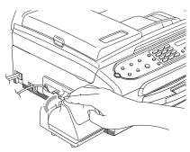
6 Route the AC power cord through the guide on the side of the machine.
