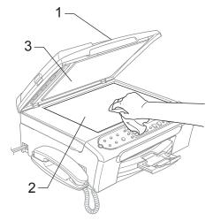
In the ADF unit, clean the white bar (1) and the glass strip (2) under it with isopropyl alcohol on a lint-free cloth.
