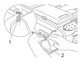
Pull the tab (1) back and hold it in position as you push the bracket (2) to the back of the machine.
