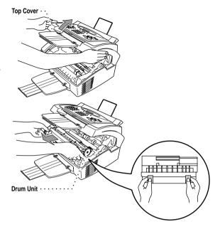
Place the drum unit on a drop cloth or large piece of disposable paper to avoid spilling and scattering the toner.
