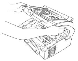
3 Holding the drum unit by its handles, insert it into the FAX/MFC.
