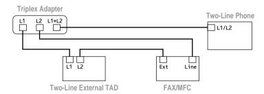
You can keep two-line telephones on other wall outlets as always. There are two ways to add a two-line telephone to the FAX/MFC's wall outlet. You can plug the telephone line cord from the two-line telephone into the L1+L2 jack of the triplex adapter. Or, you can plug the two-line telephone into the TEL jack of the two-line TAD.
