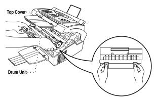
**3** Remove the toner cartridge from the drum unit and keep it in a safe place. For more information, see Replacing the Toner Cartridge, page 11-20.
