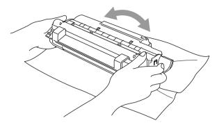
To prevent damage to the drum, do NOT expose it to light for longer than a few minutes.
