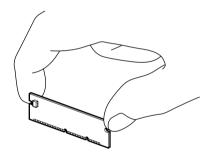
■ Make sure the memory board is securely seated on the main controller board.
