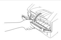
3 Insert the drum unit assembly into the machine.
