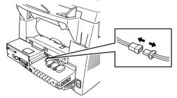
5 To install the memory board onto the main controller board, plug the attached spacer into the connectors of the main controller board.
