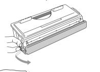
6 Install the new toner cartridge into the drum unit until it clicks into place.
