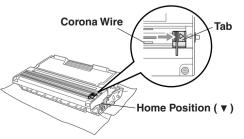
Reinstall the drum unit and close the front cover.
