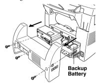
3 Remove the screws securing the access plate and remove the plate.
