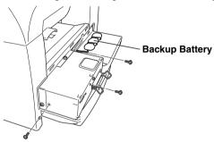
4 Disconnect the connector from the backup battery.
