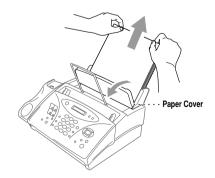
2 Open the front cover, and then open the top cover by pressing the blue levers on both sides of the top cover.
