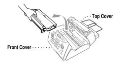
Remove the plastic stopper from the new print cartridge.
