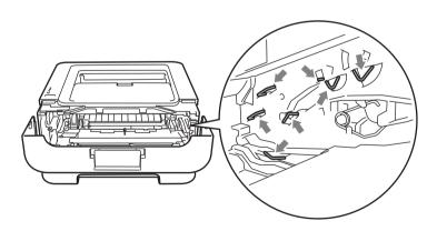
4 Put the protective material in the machine with the "REMOVE" text to the left, as shown in the illustration.
