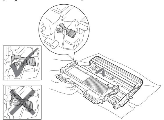
9 Open the front cover. Put the drum unit and toner cartridge assembly back into the machine.
