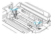
Install the Oil Bottle into the Fusing Unit with the label side facing the front of the printer.
