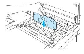
Set the Fuser Cleaner into the Fusing Unit with the roller side facing you.
