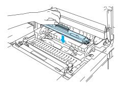
Lock the Oil Bottle and the Fuser Cleaner in place by turning the Oil Bottle Lock Levers. Close the Top Cover.
