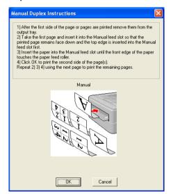
When printing to the Back output tray put the paper back in the tray in the opposite order it came out.
