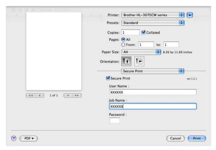
**Secure Print**: Secure documents are documents that are password protected when they are sent to the printer. Only the people who know the password will be able to print them. Since the documents are secured at the printer, you must enter the password using the control panel of the machine to print them.
