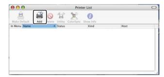
6 Choose the printer name and make sure that **Brother** is shown in **Printer Model** (**Print Using**). Select the printer name that shows **BR-Script** in the **Model Name** (**Model**), and then click **Add**.
