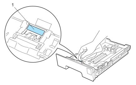
4 Wipe the two pick-up rollers (1) inside of the printer to remove dust.
