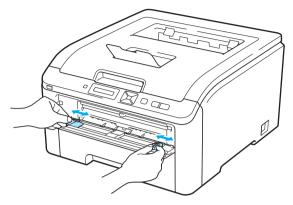
4 Using both hands, put one piece of paper in the manual feed slot until the front edge of the paper touches the paper feed roller. Wait until the machine automatically feeds the paper. When you feel the machine pull in the paper, let go.
