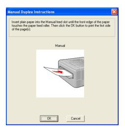
5 Remove the printed even-numbered pages from the output tray and then, in the same order <sup>1</sup>, put them back into the manual feed slot. Put the paper with the side to be printed on (the blank side) face up. Follow the instructions on the computer screen.
