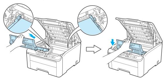
8 Slide each drum unit and toner cartridge assembly into the printer. Make sure that you match the toner cartridge color to the same color label on the printer. Repeat this for all the drum unit and toner cartridge assemblies.
