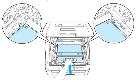
Put the belt unit back in the printer.
