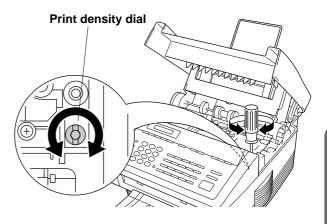
Use a straight blade screwdriver to turn the print density dial clockwise for darker print and counterclockwise for lighter print. The dial has been set to the middle position.
