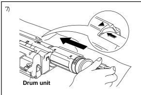
7) Slide the new toner cartridge into the opening on the right hand side of the drum unit. To ensure that the toner cartridge and the drum unit fit together correctly, make sure that the toner cartridge guide bar is exactly aligned with the guide slot in the drum unit.
