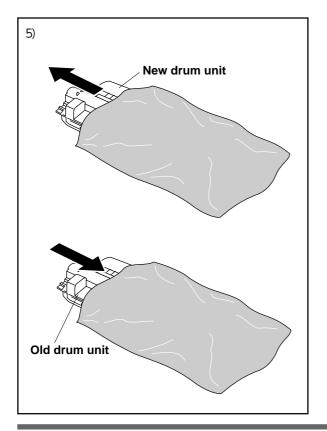
5) Wait to unpack the new drum unit until immediately before installing it. Place the old drum unit into the aluminum bag and discard it according to local regulations.
