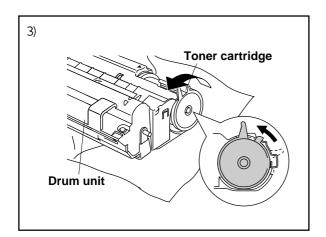
3) Gently turn the lever on the toner cartridge forward until it stops. The toner cartridge can not be removed unless the shutter is completely closed, by turning the lever fully to the front.
