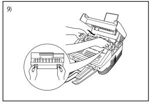
9) Reinstall the drumunit into the MFC and close the top cover. Then, turn on the power switch or plug in the power cord.
