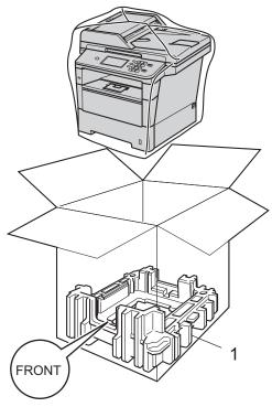
5 Put the packing material (2) marked "RIGHT" on the right of the machine. Put the packing material (3) marked "LEFT" on the left of the machine. Put the AC power cord and printed materials in the original carton as shown in the illustration.
