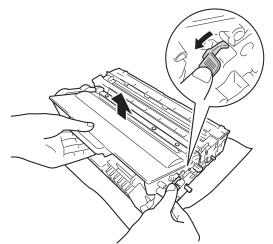
1 Turn the drum unit as shown in the illustration. Make sure that the drum unit gear (1) is on the left hand side.
