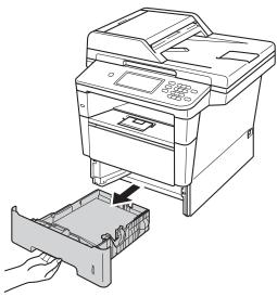
4 Tightly wring out a lint-free cloth soaked in lukewarm water, and then wipe the separator pad (1) of the paper tray with it to remove dust.
