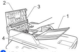
Lift the document cover (1). Clean the white plastic surface (2) and scanner glass (3) underneath it with a soft lint-free cloth moistened with water.
