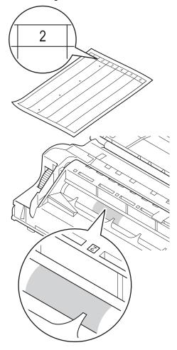
**1**3 Turn the drum unit gear toward you by hand while checking the surface of the suspected area.
