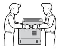
If you use a Lower Tray, DO NOT carry the machine with the Lower Tray as you may be injured or cause damage to the machine because it is not attached to the Lower Tray.
