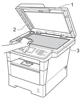
In the ADF unit, clean the white bar (1) and the glass strip (2) underneath it with a soft lint-free cloth moistened with water.
