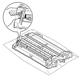
When you have found the mark on the drum that matches the drum dot check sheet, wipe the surface of the drum gently with a cotton swab until the mark on the surface comes off.
